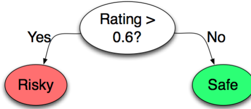
Figure 3: Example of a stump classifier. A stump classifier is a machine-learning model consisting of a one-level decision tree. A decision stump makes a prediction based on the value of a just single input feature.
