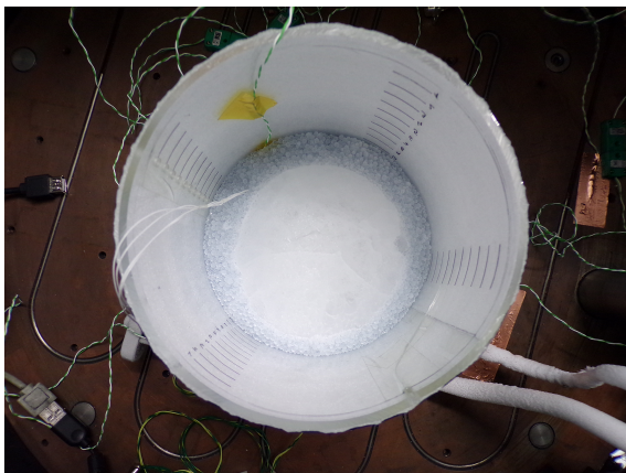
Figure 2. Setup for our CO 2 ice measurements. The cooling plate is connected via the pipes shown in the right lower corner to a LN 2 Dewar and a digital temperature control unit to stabilize the temperature. The image was taken after the measurements were done.
